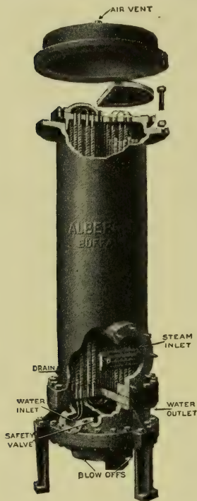
FIG. 19.—Alberger Vertical Feed-Water Heater
